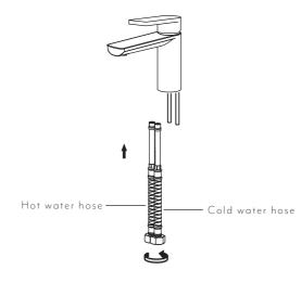
Install the basin mixer by fixing the washers, nut & screws on the underside of the benchtop.
