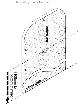
Mount mirror to wall by lining up mirror with marked position on wall & fastening brackets together with cable fastener provided.
