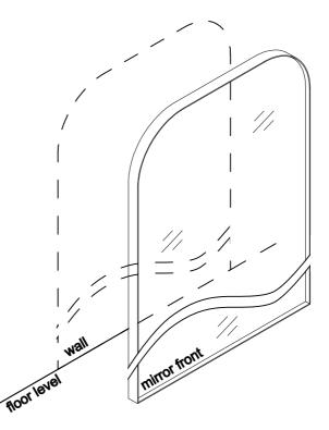
Position the wall fixing brackets with measurements taken from the mirror bracket positions. Using the screws provided fix wall brackets into structural support in wall.
