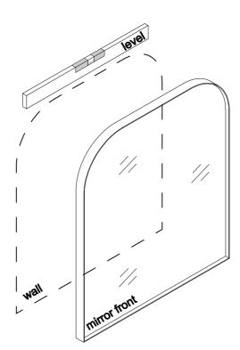
Position the wall fixing brackets with measurements taken from the mirror bracket positions. Using the screws provided fix wall brackets into structural support in wall.
