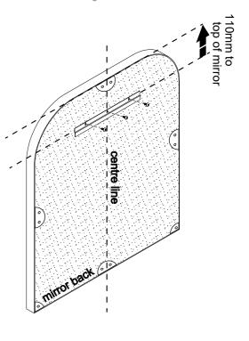
Mount mirror to wall by lining up mirror with marked position on wall & lowering the mirror brackets into wall brackets.
