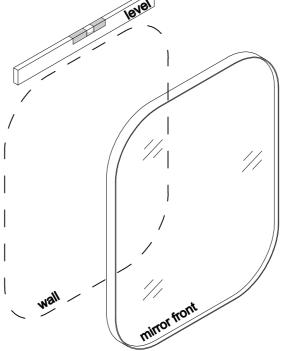
Position the wall fixing brackets with measurements taken from the mirror bracket positions. Using the screws provided fix wall brackets into structural support in wall.
