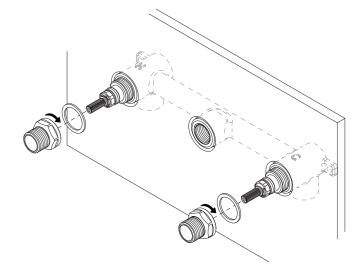
Remove locking nut from spindle. Screw spindle into breach and hand tighten until rear of spindle meets the body seat, be sure not to over tighten. If necessary apply more pressure lightly with spanner.
