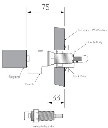
For distances 65mm up to 75mm between nogging and finished wall surface, an extended spindle is required. Set back from handle body to backplate will be decreased as wall cavity increases.
