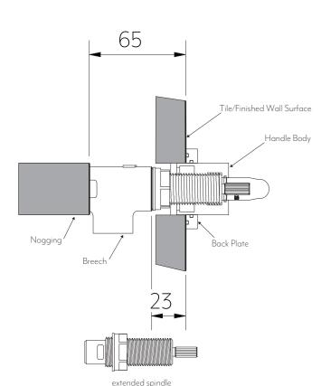
For installations when distance between nogging and finished wall surface is 65mm, and a larger set back from handle body to back plate is preferred, an extended spindle can be used (available for additional purchase).
