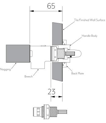
In the instance of a thicker finished wall surface, to achieve a distance of 45mm to 65mm from nogging to finished wall surface a standard spindle can continue to be used, however spacing from handle body to back plate will be decreased.
