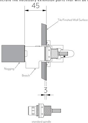
Minimum distance between nogging and finished wall surface is 45mm (or 3mm from in-wall breech to finished wall surface).
