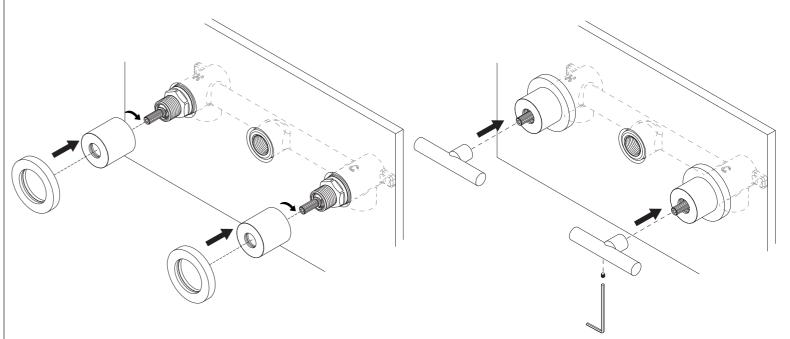
Install the handle body onto the locking nut, twisting by hand until tightened. Slide back plate over handle body until firmly pressed against finished wall surface.
