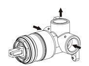
Push the sleeve over the body until it is as far back as possible and nut thread is exposed. Screw the dome onto the brass fitting and tighten.
