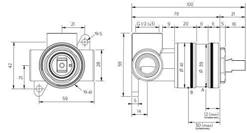
Disclaimer: To achieve Infiniti (interchangeable sleeves) finish wall must fall between Point A and B. Your In-Wall component must be installed without the sleeve attached, please ensure that your chosen sleeve doesn't break your waterproofing seal.
