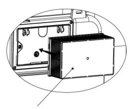
Plastic holder (to reserve space for installation actuator at wall building. To prevent dust impurities into tank at wall building)
