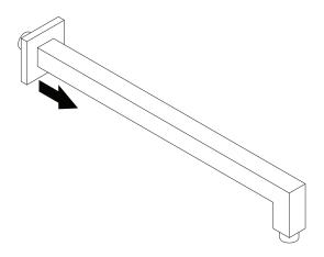
Apply the teflon tape to the brass nipple. Twist the spout on and hand tighten. Push back plate to the wall surface.
