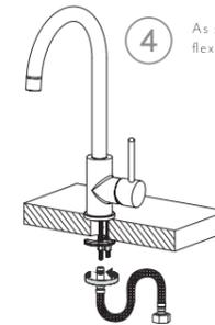
5 Attach the two flexible hoses to water supply
