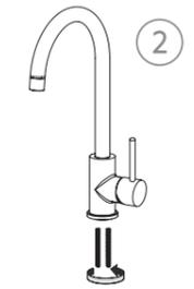
3 Put the faucet into the hole. Pass the horseshoe plates through the bolts, fasten the nuts and tighten
