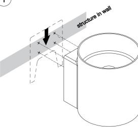
Hold basin against wall aligning outlet of trap with waste pipe. Extend telescopic trap up or down to find desired height & cut waste to suit trap.
