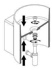
4 If correct height and position is suitable, level the top of the basin & mark out desired position.
