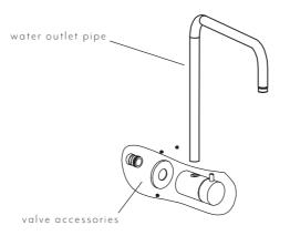
Put the straight arm into the holder, value accessories and wall seat, use M5 screws. Install the water outlet pipe into the top.
