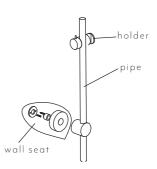
Before installing shower head, open and clean the pipe. Put the flow rate limiter and gasket into the shower head, then connect the shower head with the water outlet. Screw the head.
