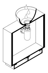
2 Install pop up waste and attach to plumbing. Test by running water through the waste and pushing the plug down.
