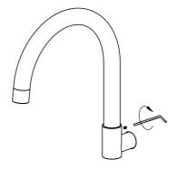
Rotate the body onto the water outlet (1/2 inch nipple) with teflon tape and firmly
