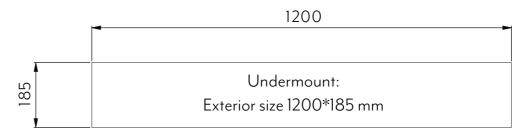
UNDERMOUNT INSERT TEMPLATE- refer to install method 3
