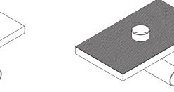
Cut PVC pipe 3mm below tile finish face.
