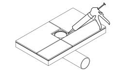
Press Inspection outlet into recess, ensuring it is level with tile finish face.
