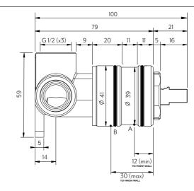
Disclaimer: To achieve infiniti (interchangeable sleeves) finish wall must fall between Point A and B
