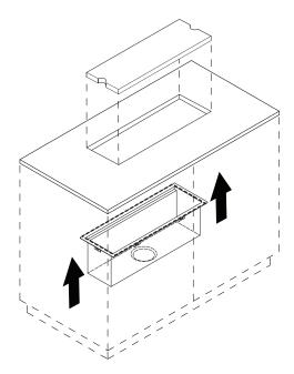
Undermount Fixing Detail
