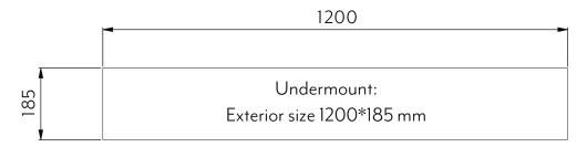
UNDERMOUNT INSERT TEMPLATE- refer to install method 3
