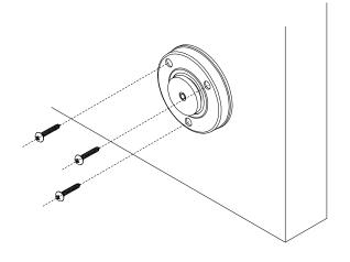
Fix stop to floor using fixings provided.
