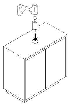
Mark out desired location of basin and drill hole for basin waste with a hole saw.
