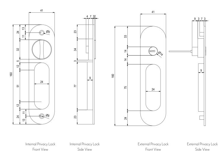
Designed for internal doors of thickness 45-60mm. Not suitable for Australian or New Zealand standard internal doors.
