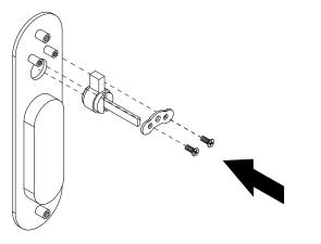
Adjust coin lock extension by cutting with tin snips or hacksaw to suit door thickness.
