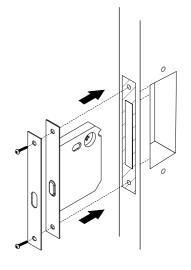
Fix front and back panels to latch.
