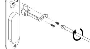
Note: The 16mm screw option is required (supplied with 30-50mm coin lock set) in order to suit a 35mm Australian standard door.
