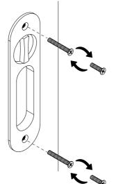
Fix coin lock to the frame. Ensure the bracket and key is oriented with the peak directed up (as illustrated).
