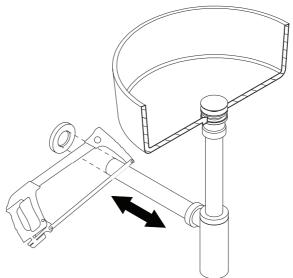
Assemble trap and tighten all components.
