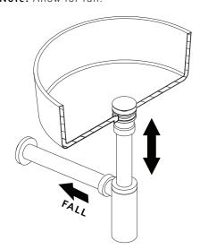
Engage kee seal into 40mm socket.
