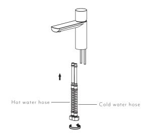
Attach the two flexible hoses to water supply and hand tighten. Remove the aerator from the spout and flush.
