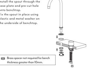
Attach spout to mixer using flexible hose.
