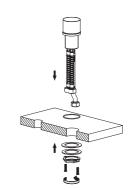
Install the spout through the base plate and pre-cut hole onto benchtop.
