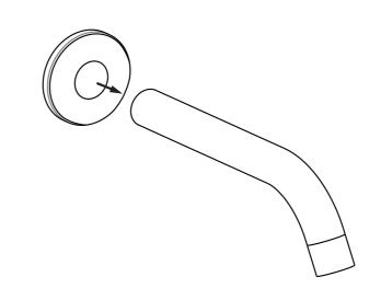
Apply the teflon tape to the brass nipple.
