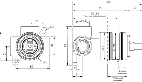
Disclaimer: To achieve Infiniti (interchangeable sleeves) finish wall must fall between Point A and B. Your In-Wall component must be installed without the sleeve attached, please ensure that your chosen sleeve doesn't break your waterproofing seal.
