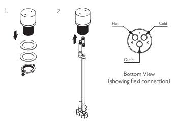
Attach the hot/cold flexi hoses to the corresponding hot/cold water supply.
