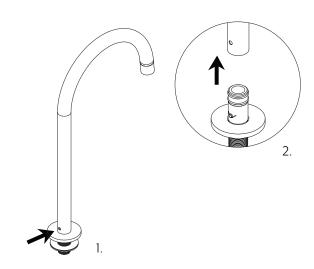
Fix base connection to benchtop with brass nut ensuring the rubber washer and spacer are fitted to the underside of the benchtop.
