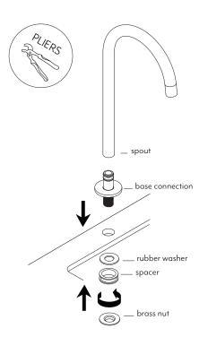
(4) Connect pipework to inlet of spout.
