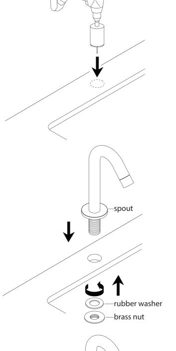
Fix spout to benchtop with brass nut ensuring rubber washer is fitted to underside of benchtop.
