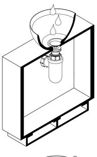
2 Install pop up waste and attach to plumbing. Test by running water through the waste and pushing the plug down.
