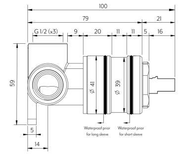
Disclaimer: To achieve infiniti (interchangeable sleeves) waterproofing can not exceed past sleeve B.
