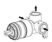
Push the sleeve over the body until it is as far back as possible and nut thread is exposed. Screw the dome onto the brass fitting and tighten.
