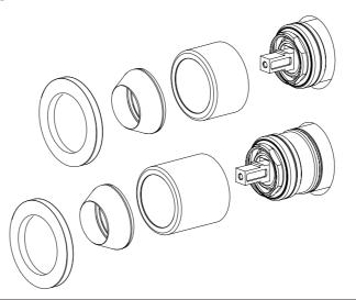
Create a 47mm hole in cement sheet (3)Waterproof at this point if future sleeve change is desired. DO NOT WATERPROOF SLEEVE.
