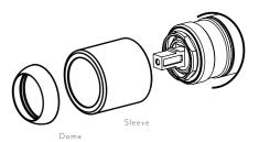
\*Please ensure that the hole is big enough to allow for the sleeve to slide on at fit-off stage\*
