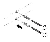
a. Screw spacers into the back of singage.
