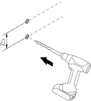
For easy install place threaded rod into drill. Where the thread changes marks approx 6mm. Drill the rod straight into the sub-straight or anchors and undo the chuck leaving the rod protruding from the wall 6mm. Minor adjustments can be made with a small phillips head screwdriver.
