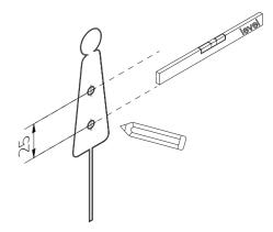
If required insert wall anchors into predrilled holes and screw threaded rods into the anchors leaving approx. 6mm of the rod protruding from the wall.
