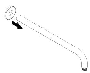
Apply the teflon tape to the brass nipple. Twist the spout on and hand tighten. Push back plate to the wall surface.
