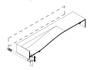
Secure plumbing to basin and wall outlet. Test by running water through the waste. Silicon top and sides of basin if necessary.
