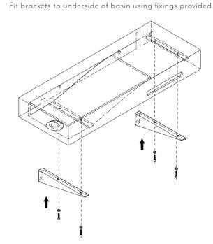
Hold basin against wall aligning outlet of trap with waste pipe. Extend telescopic trap up or down to find desired height & cut waste to suit trap.
