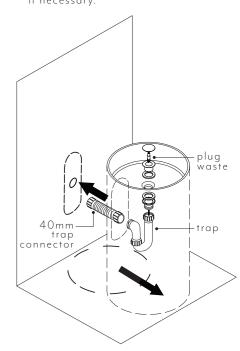
Fit plug waste into basin outlet, seal & tighten as required.
