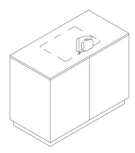
Lay a peice of timber across the benchtop hole & position (3)in line with sink hole below.
