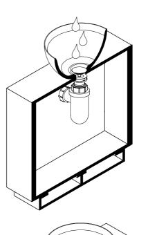
Install pop up waste and attach to plumbing. Test by running water through the waste and pushing the plug down.
