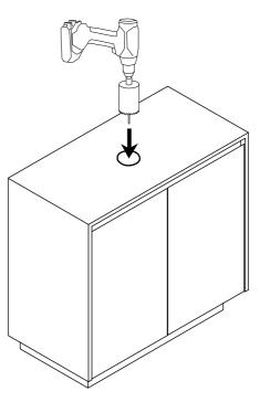
Mark out desired location of basin and drill hole for basin waste with a hole saw.
